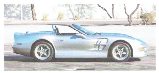
**Dimensions:** Length; 169.0" (4,292 mm). Width; 76.5" (1,943 mm). Height; 47.0" (1,194 mm). Weight; 2,650 lb (1,202 kg) – (Note: weight of actual production cars varied up to almost 3,000 lb with a full tank of fuel depending on the weight of the body panels: likely to be heavier on early production cars and lighter on late production cars).
